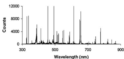
Figure 2. Typical LIBS spectrum
