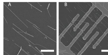
We use photolithography to pattern microfabricated electrodes for transport measurements on semiconductor nanowires, and to pattern microfluidic structures for in-situ measurements.
