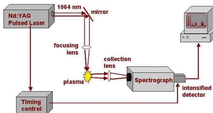
Figure 1. Block diagram of LIBS experiment
