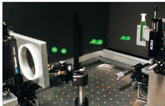
Fig. 1. New methods using the coordinated action of six, ultrafast laser pulses can separate the dynamics of different molecular subensembles within a heterogeneous sample. The pulses (green) have passed through the lens on the left and are being focusing onto a common point in the sample (green cuvette) on the right.
