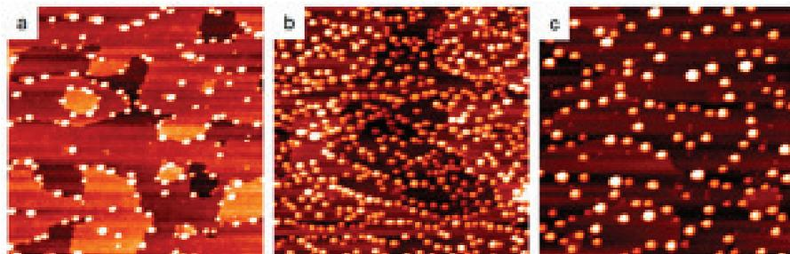
Figure 1: STM images of Au and Au-Ni nanoparticles on  $\text{TiO}_2$ . See text for more details. All images are  $100 \times 100 \text{ nm}^2$
