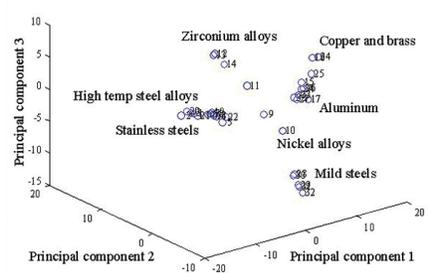
Figure 3. Identification of alloys by principal component analysis of their LIBS spectra
