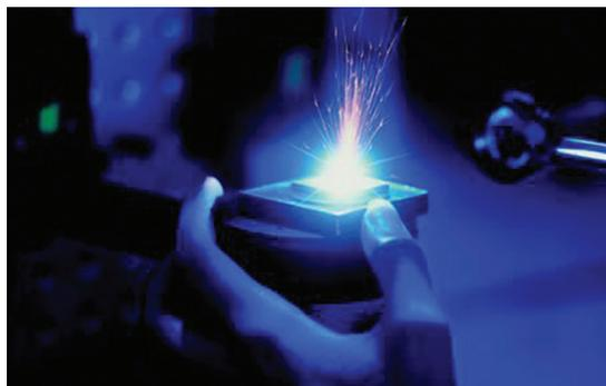
In LIBS, the sample is ablated and ionized using a pulsed laser. Analysis of the emission from the plasma provides information on the elemental composition of the sample. This technique is unique in that elemental composition can be determined remotely.
